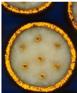
Fig.1. The image shows is camphor layer contained in the Phlegmatic propellant
