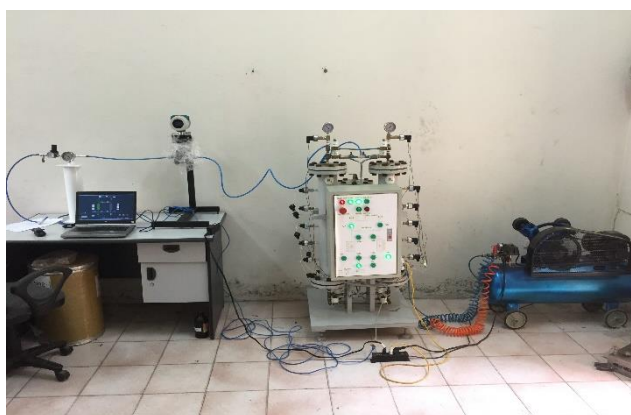
Fig. 3. The nitrogen gas generator working follow pressure swing adsorption
